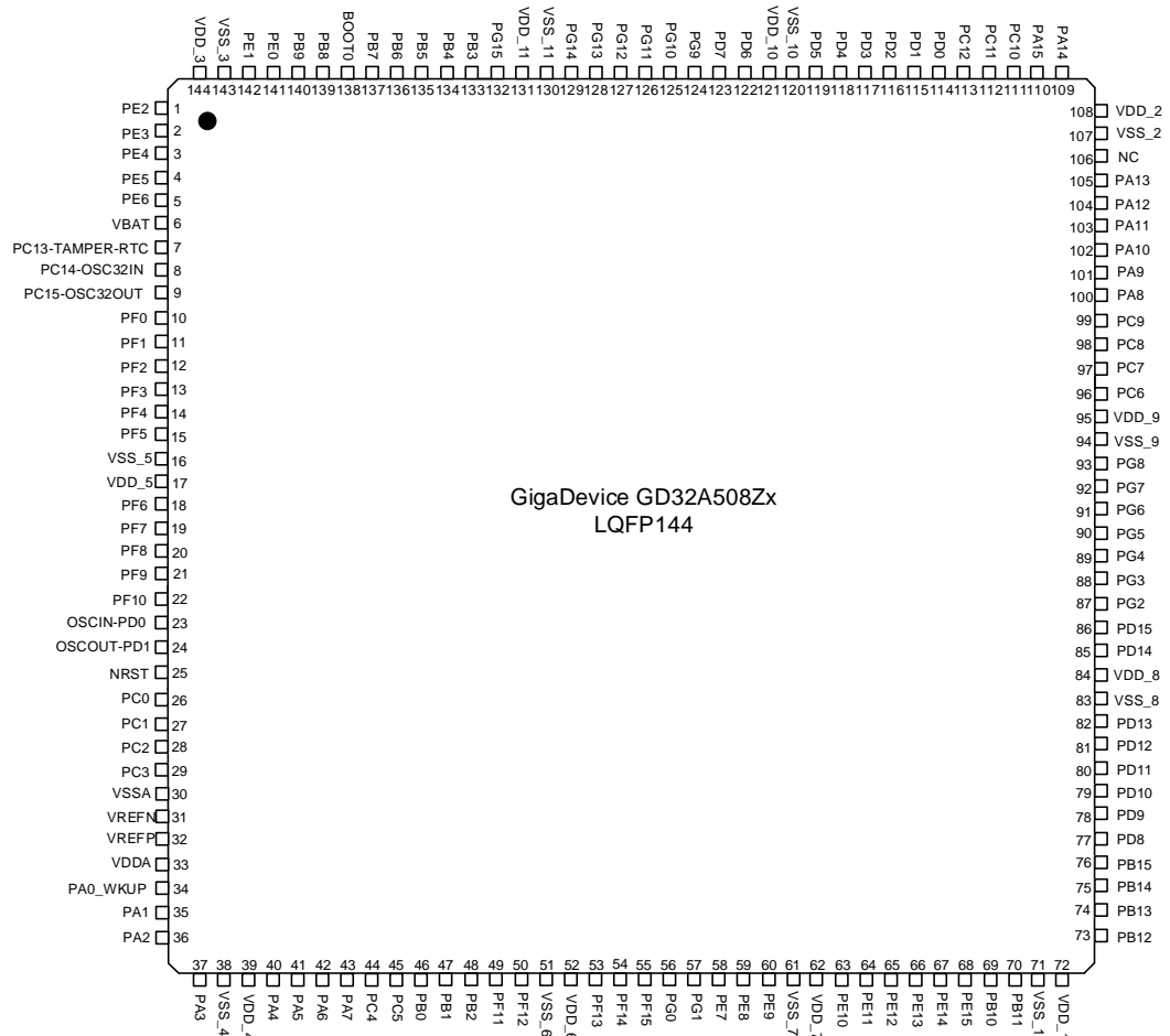
Figure 2-2. GD32A508Zx LQFP144 pinouts
