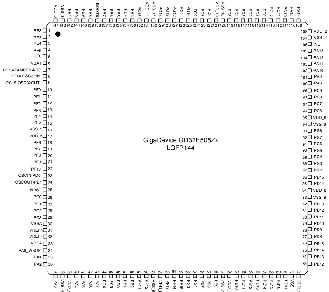
Figure 2-2. GD32E505Zx LQFP144 pinouts
