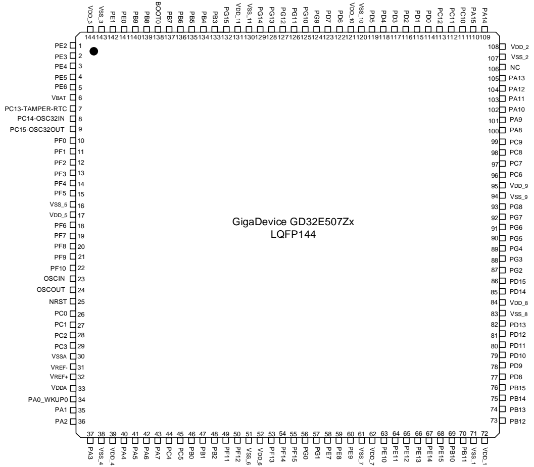
Figure 2-2. GD32E507Zx LQFP144 pinouts
