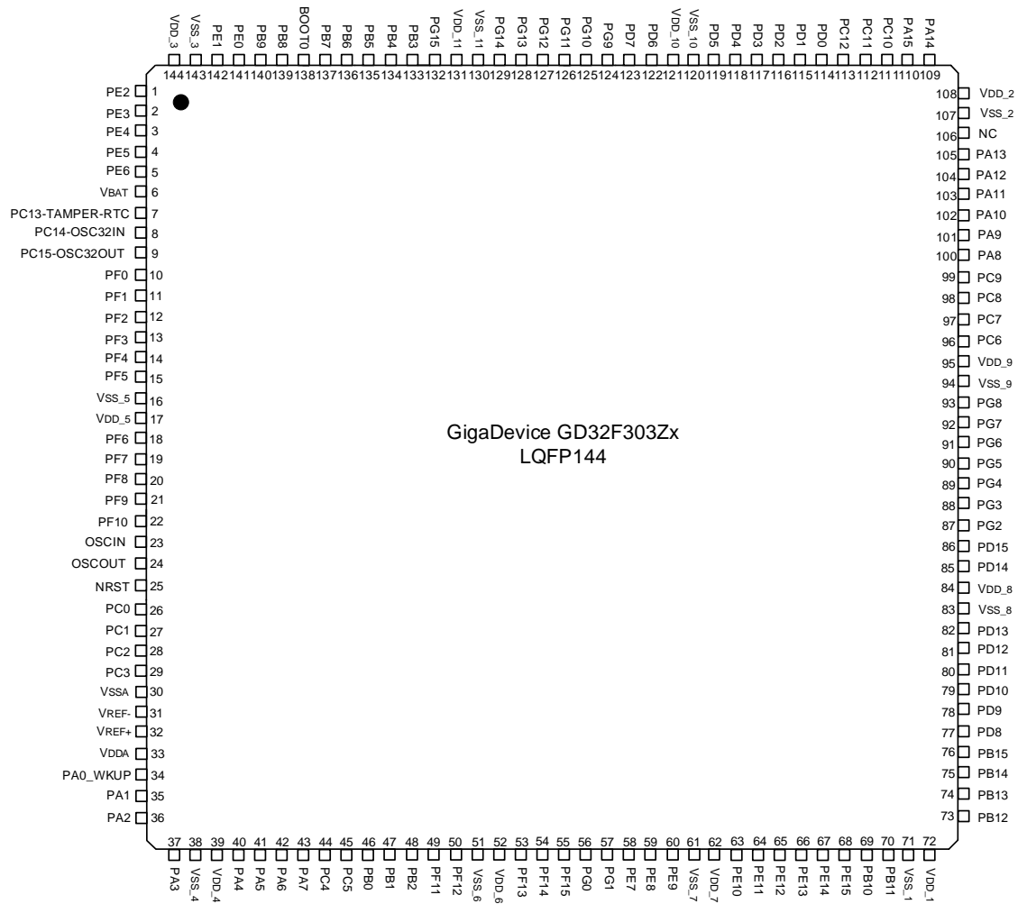
Figure 2-2. GD32F303Zx LQFP144 pinouts
