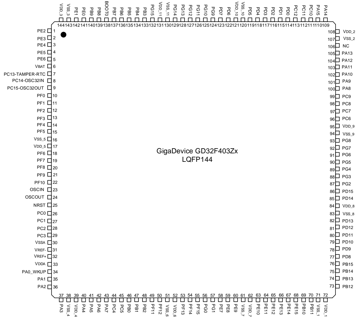
Figure 2-2. GD32F403Zx LQFP144 pinouts
