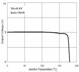
**Output Voltage vs Junction Temperature**
