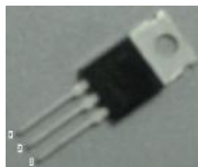
1.Gate 2.Drain 3.Source
