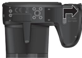
2. Insert the batteries in the correct direction by matching the + - label on the battery slot.
