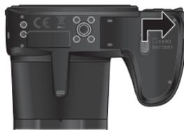
2. Insert an SD card in the correct direction.
