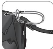
5. Attach the other end of the lens strap on the lens cover.
