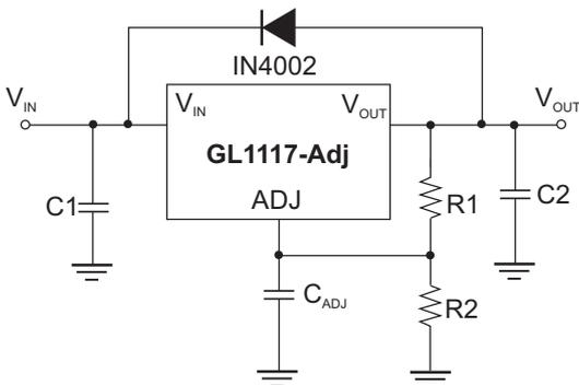
In the GL1117 linear regulators, the discharge path is through a large junction, and protection diodes are normally not needed. However, damage can occur if the regulator is used with large output capacitance values and the input voltage is instantaneously shorted to ground. In this case, a diode connected as shown above in Figure 2.
