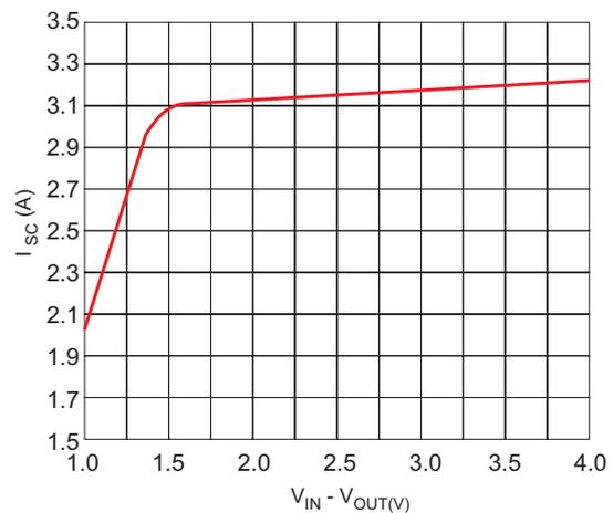
Figure 9. Short Circuit Current vs.  $V_{IN} - V_{OUT}$
