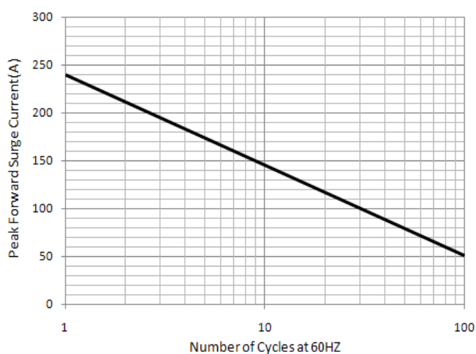
Figure 2. Maximum Non-Repetitive Peak Forward Surge Current Per Leg
