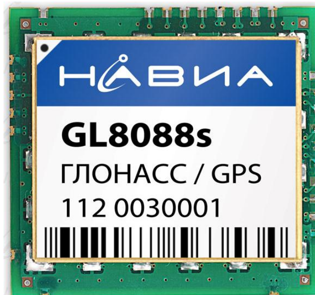
Fig. 1. The exterior view of the receiver module.
