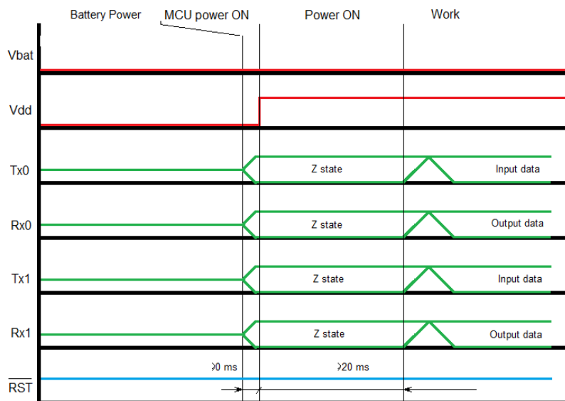
Fig. 7. The signal states and levels timing diagram at the module connection terminals when the module is used without Vbat.
