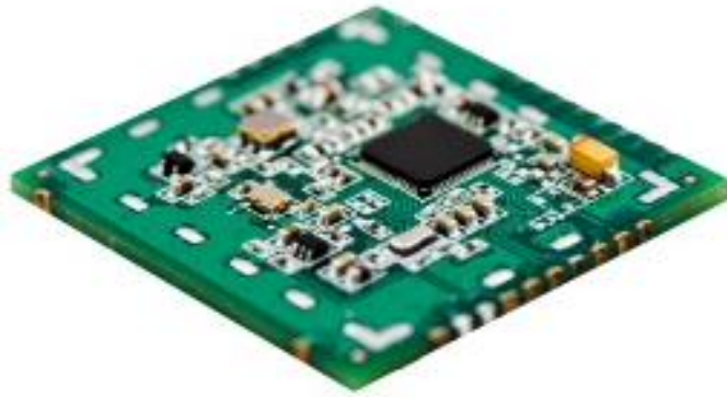
Fig. 2. View of the receiver board with the screen removed.
