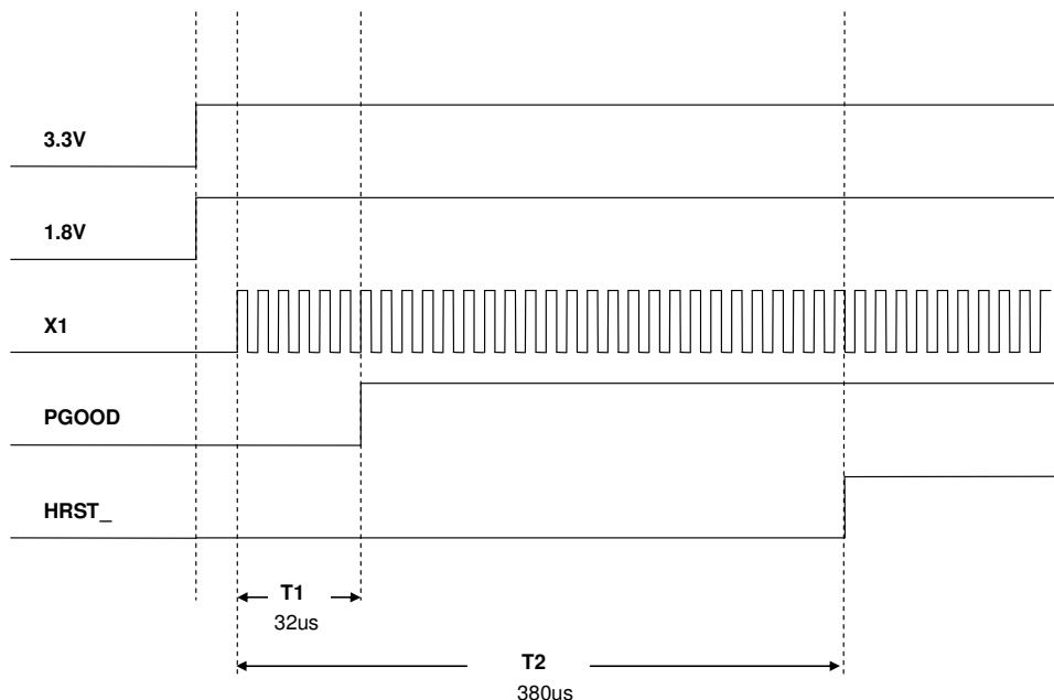
**Figure 6.1 - Reset Timing**
