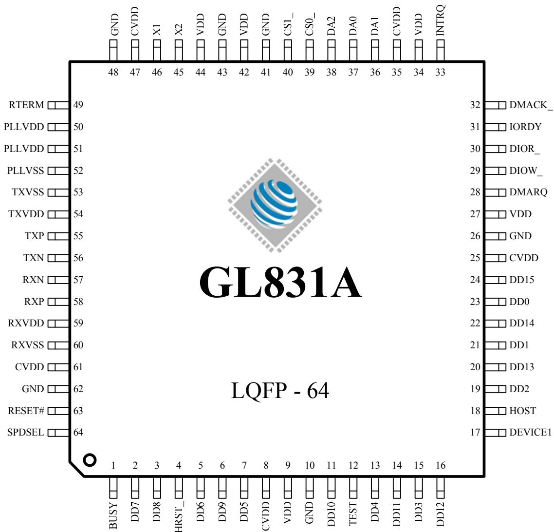
**Figure 3.1 - 64 Pin LQFP Pinout Diagram**
