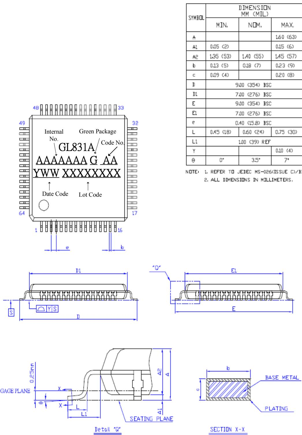
**Figure 7.1 - LQFP 64 Pin Package**
