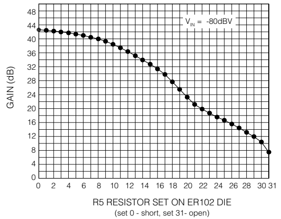
Fig. 6 High Frequency Gain (Compression Ratio Adjustment)
