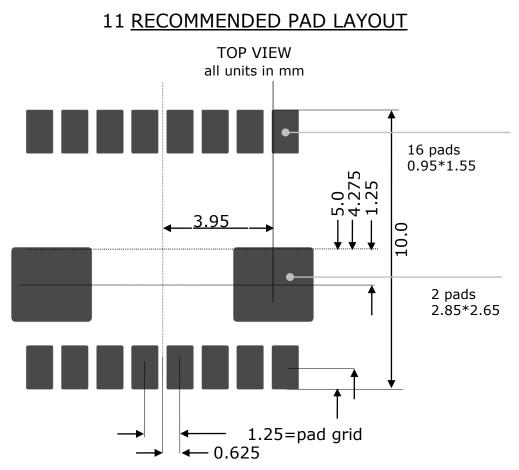
Note: For prototyping, GNS3301 is available on a stamp design adaptor board. Recommended mainboard pad layout will fit for both.
