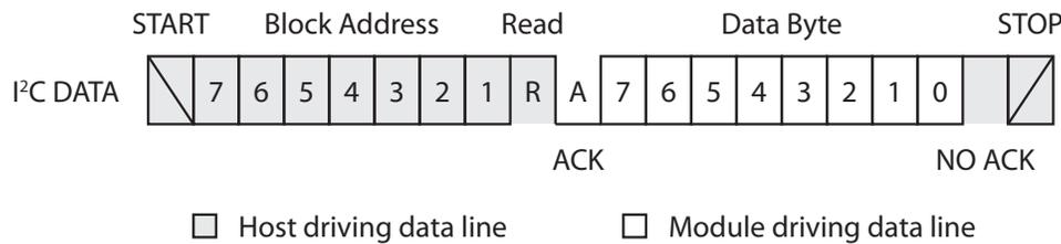
Figure 4-2: I<sup>2</sup>C Current Address Read Operation
