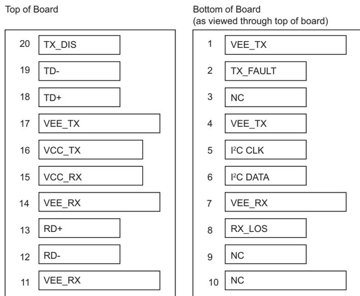
Figure 2-2: GO2921B Edge Connector Pad Configuration
