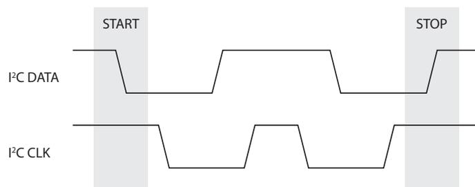
Figure 4-1: I<sup>2</sup>C START and STOP Condition
