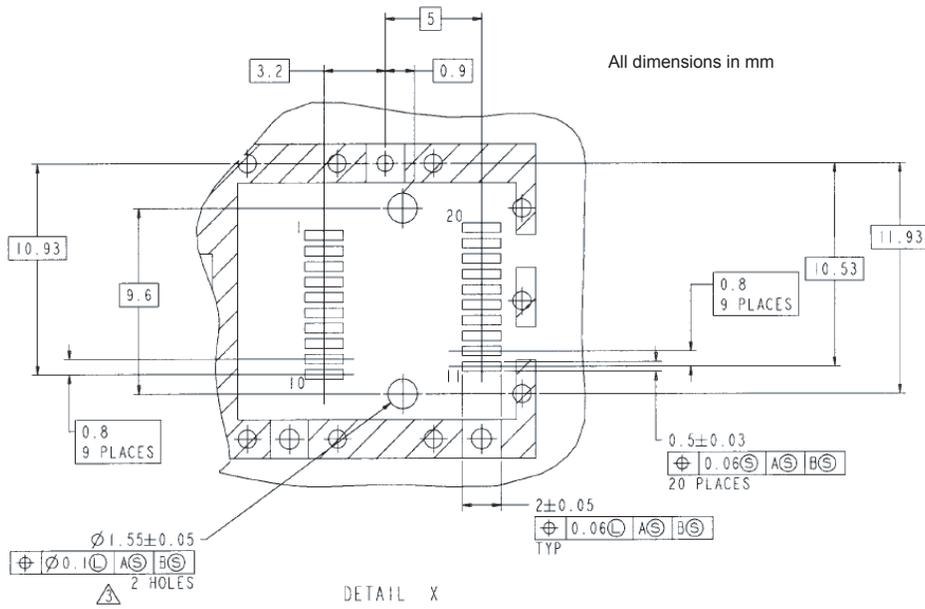
Figure 7-4: Host PCB Layout – Part 2
