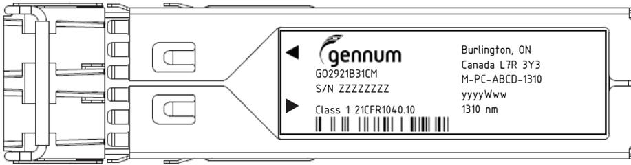
Figure 7-2: GO2921B Marking Diagram
