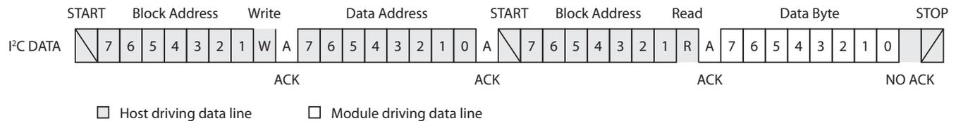
Figure 4-3: I<sup>2</sup>C Random Access Read Operation
