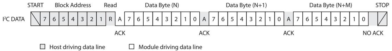
Figure 4-4: I<sup>2</sup>C Sequential Read Access Operation
