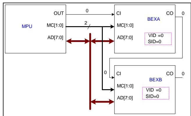
\$000DH register works for setting a unique VID for each BEXs, and then acts as SID only. VID are write-once register. The first step is accessing BEXA and then accessing BEXB as follows:
