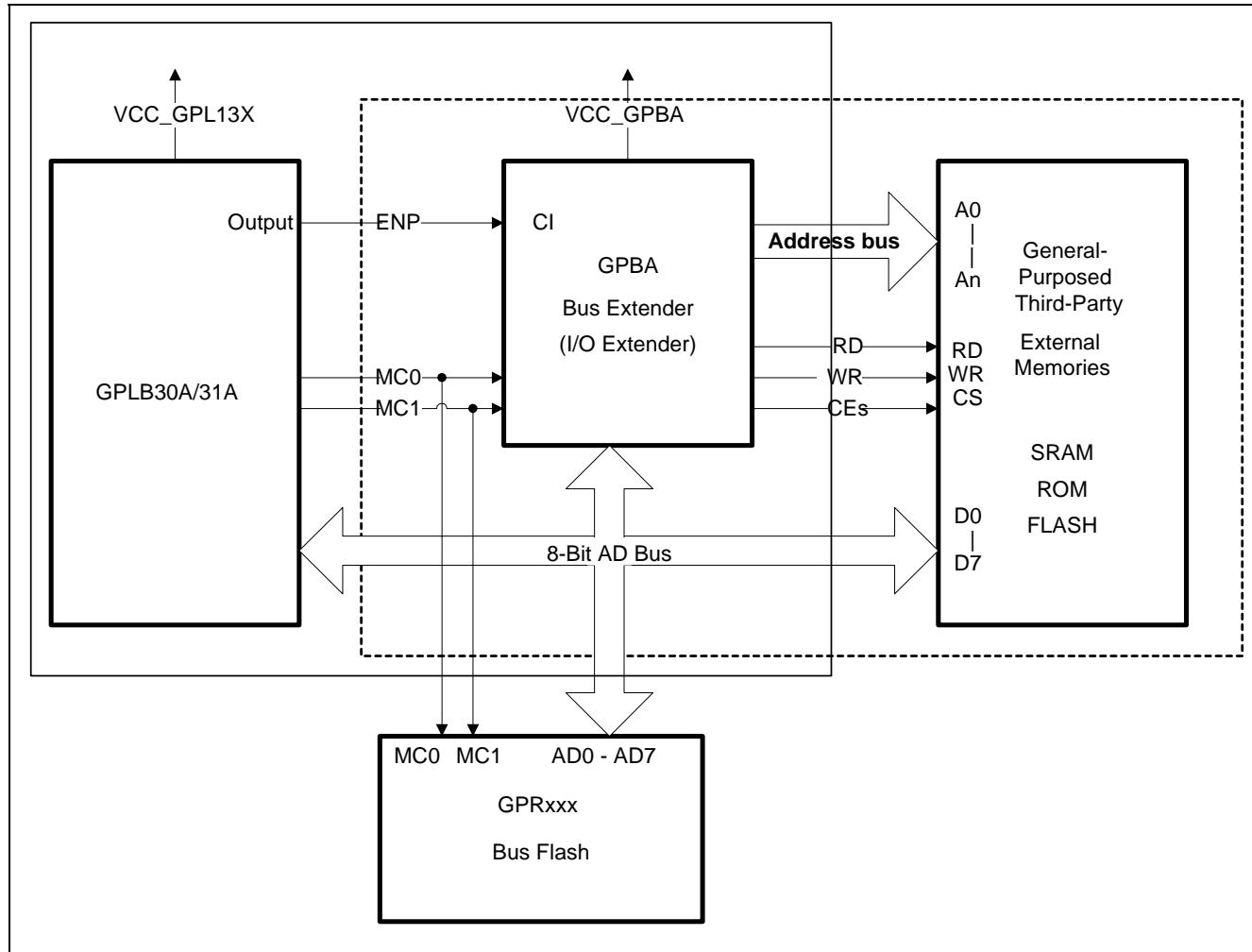
The area in solid line can be viewed as a micro-controller with address bus.
