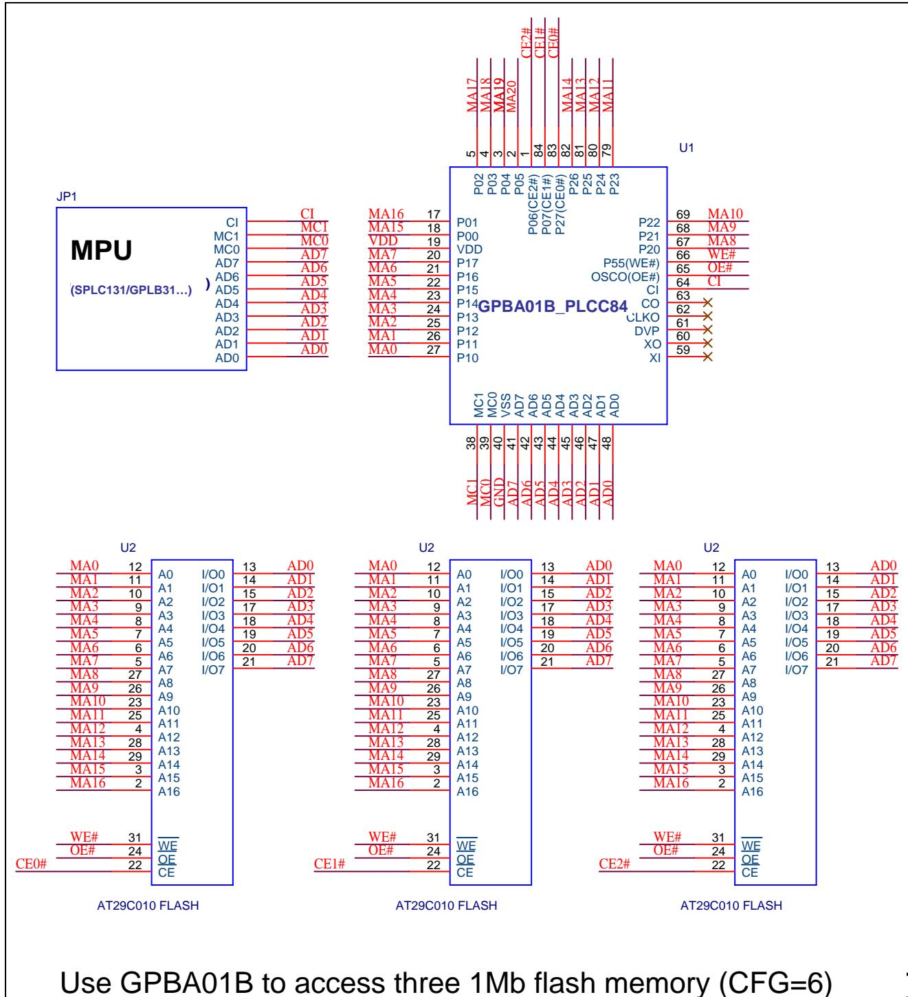
Use GPBA01B to access three 1Mb flash memory (CFG=6)
