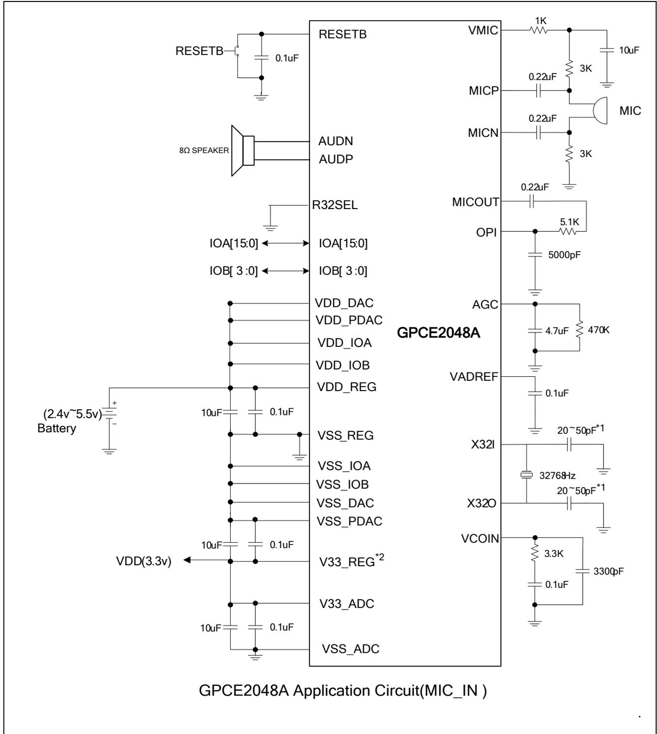
**Note1:** These capacitor values are for design guidance only. Different capacitor values may be required for different crystal/resonator used.
