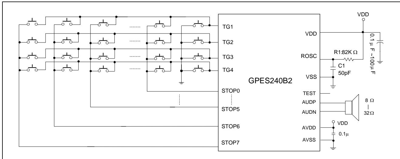
**Note:** To avoid the noise interference on PCB around R-oscillator, R1 and C1 should be placed as close as possible to ROSC pin.
