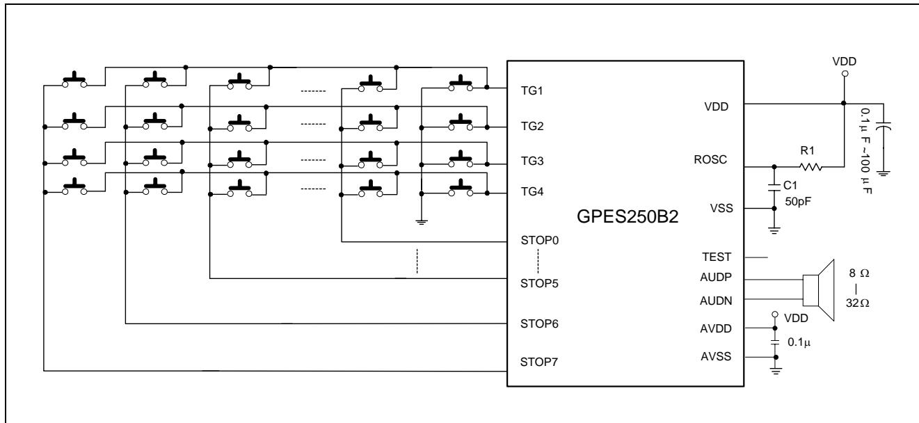
**Note:** To avoid the noise interference on PCB around R-oscillator, R1 and C1 should be placed as close as possible to ROSC pin.
