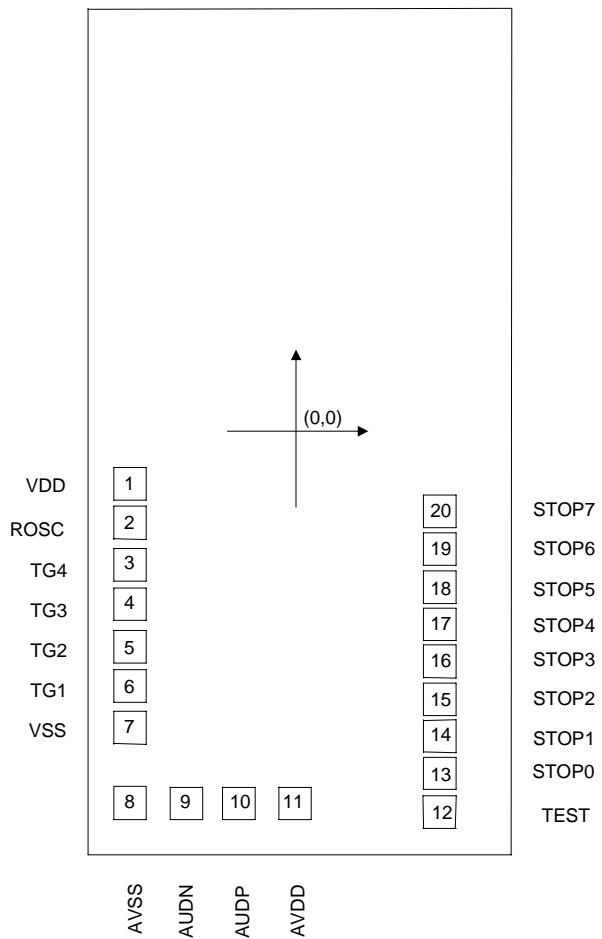
This IC substrate should be connected to VSS
