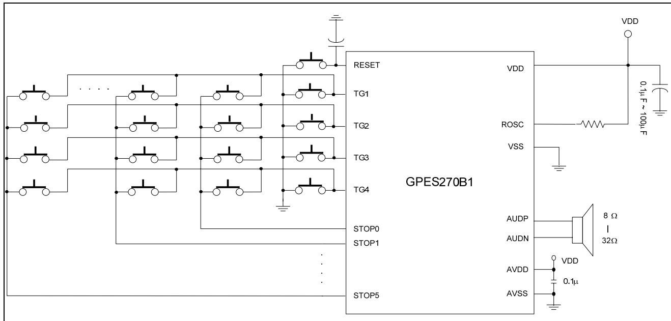
**Note:** To avoid the noise interference on PCB around R-oscillator, R1 and C1 should be placed as close as possible to ROSC pin.
