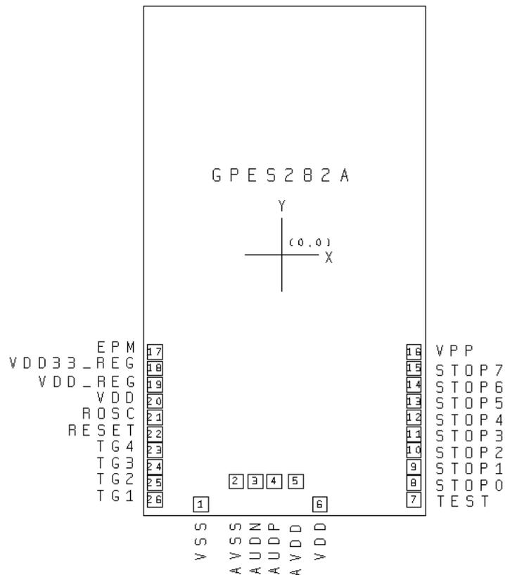
This IC substrate should be connected to VSS
