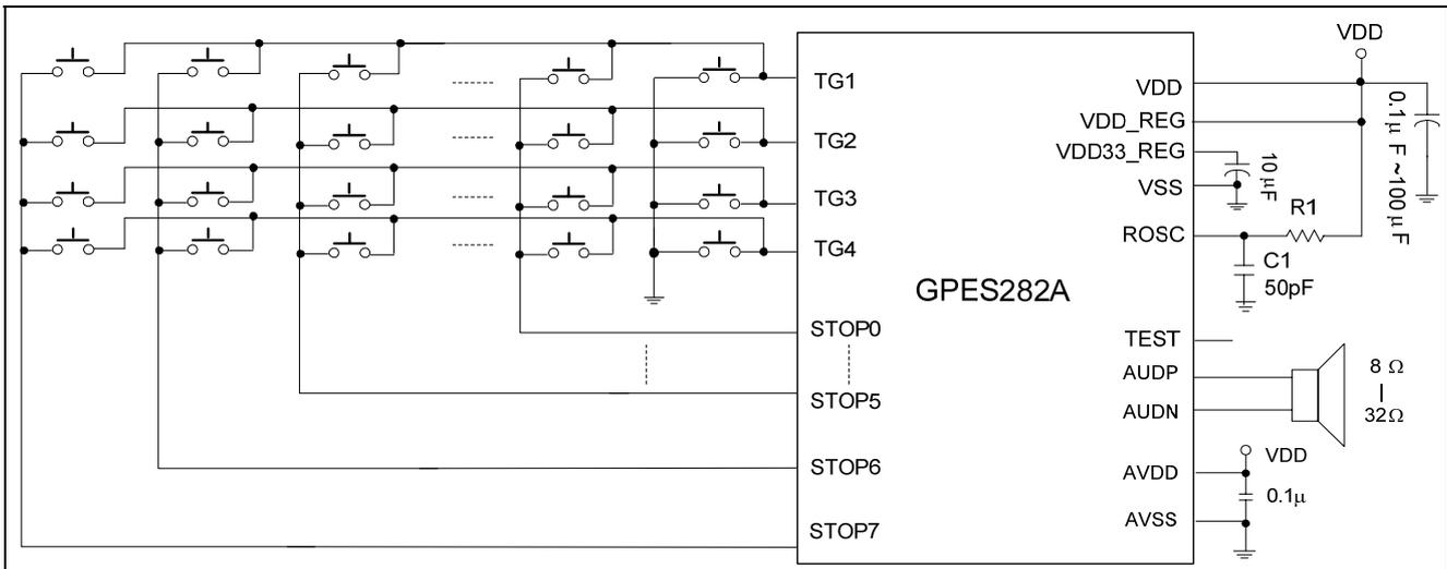
**Note:** To avoid the noise interference on PCB around R-oscillator, R1 and C1 should be placed as close as possible to ROSC pin.
