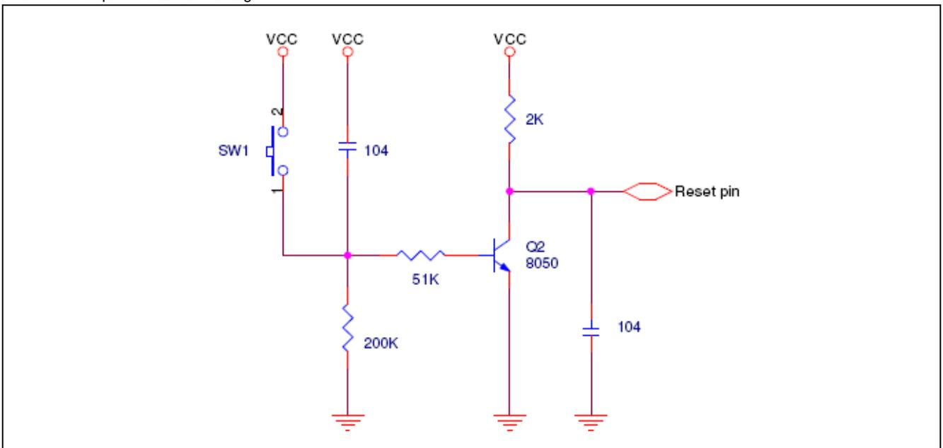
The resistor and capacitor value is depend on the switch type, please contact Generalplus FAE for detailed.
