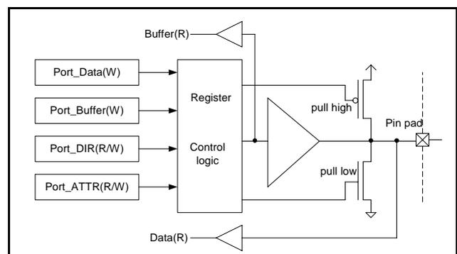
Although data can be written into the same register through Port\_Data and Port\_Buffer, they can be read from different places, Buffer (R) and Data (R). The GPIO is the key wakeup port. To activate key wakeup function, latch data on PORT Latch and
