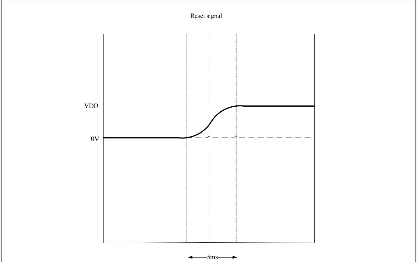
If the RESET signal is not able to achieve the above timing diagram, we suggest add the supper reset circuit in the following diagram to achieve the required RESET timing.
