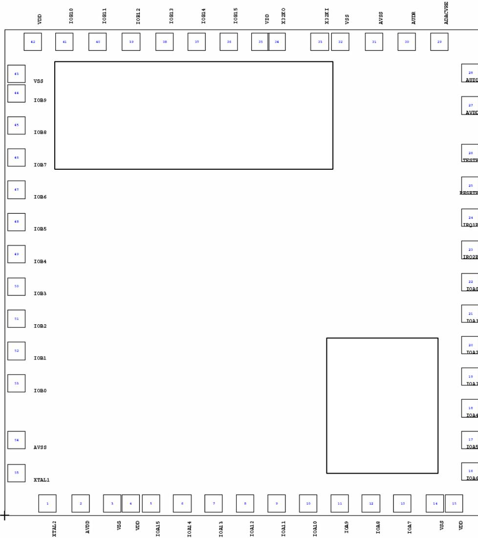
This IC substrate should be connected to VSS
