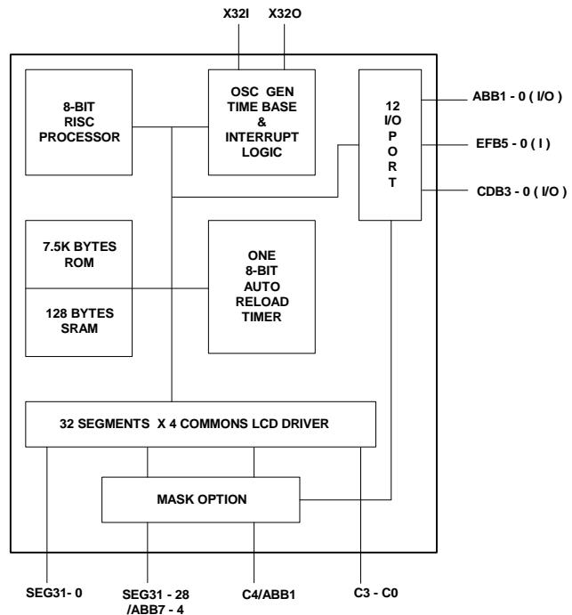
**Note1:** By mask option, SEG31 - 28 can be defined as either segment output or I/O. (SEG31 - 28 or ABB7 - 4)
