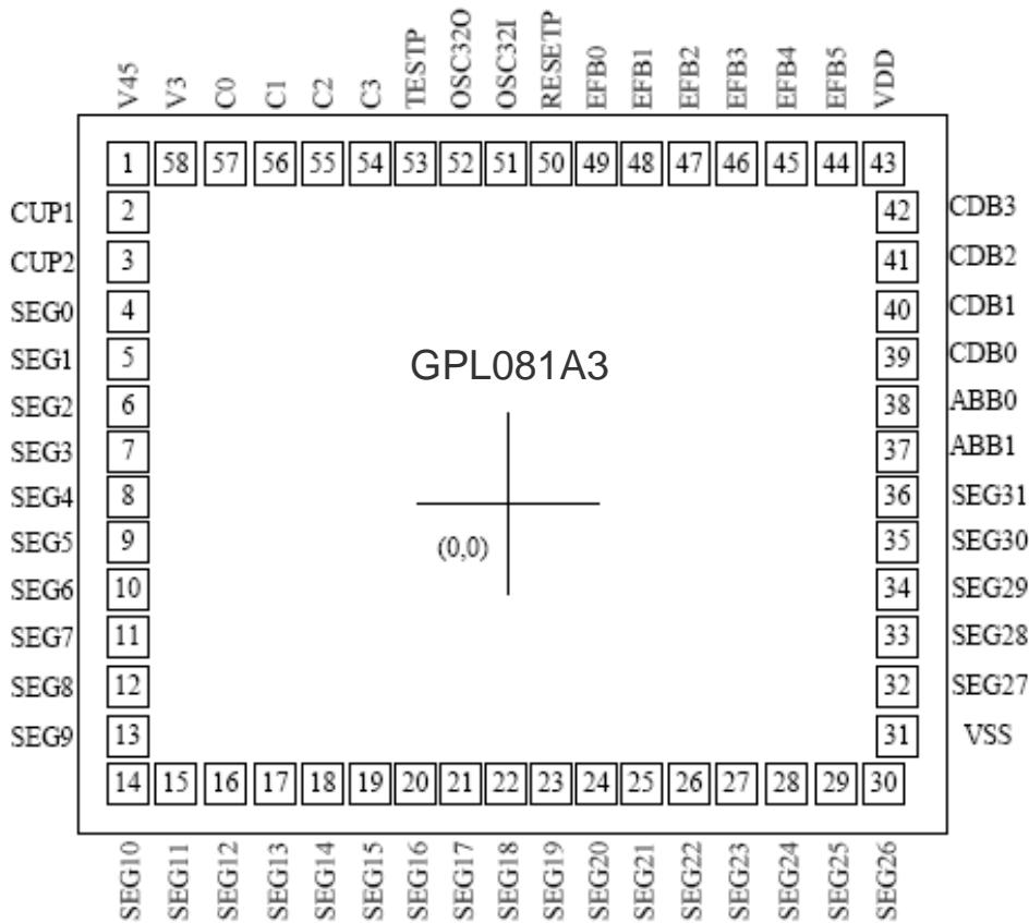
This IC substrate should be connected to VSS
