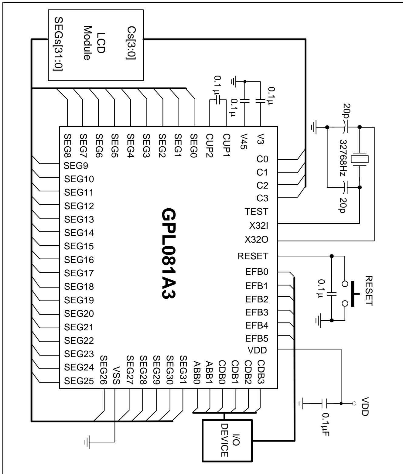
**Note:** The 0.1μF capacitor between VDD and VSS should be placed to IC as close as possible.
