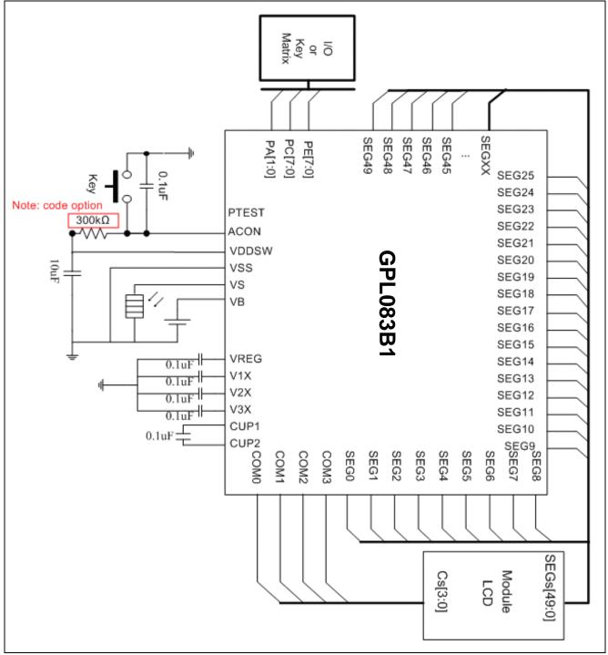
Note : The 300k $\Omega\,$  is possible to be removed, if the internal resistor is enable by code option.
