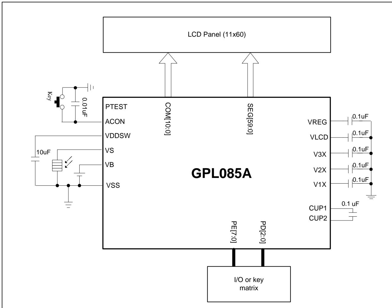
**Note1:** These capacitor values are for design reference only. Different capacitor values may be required for different crystal/resonator used.
