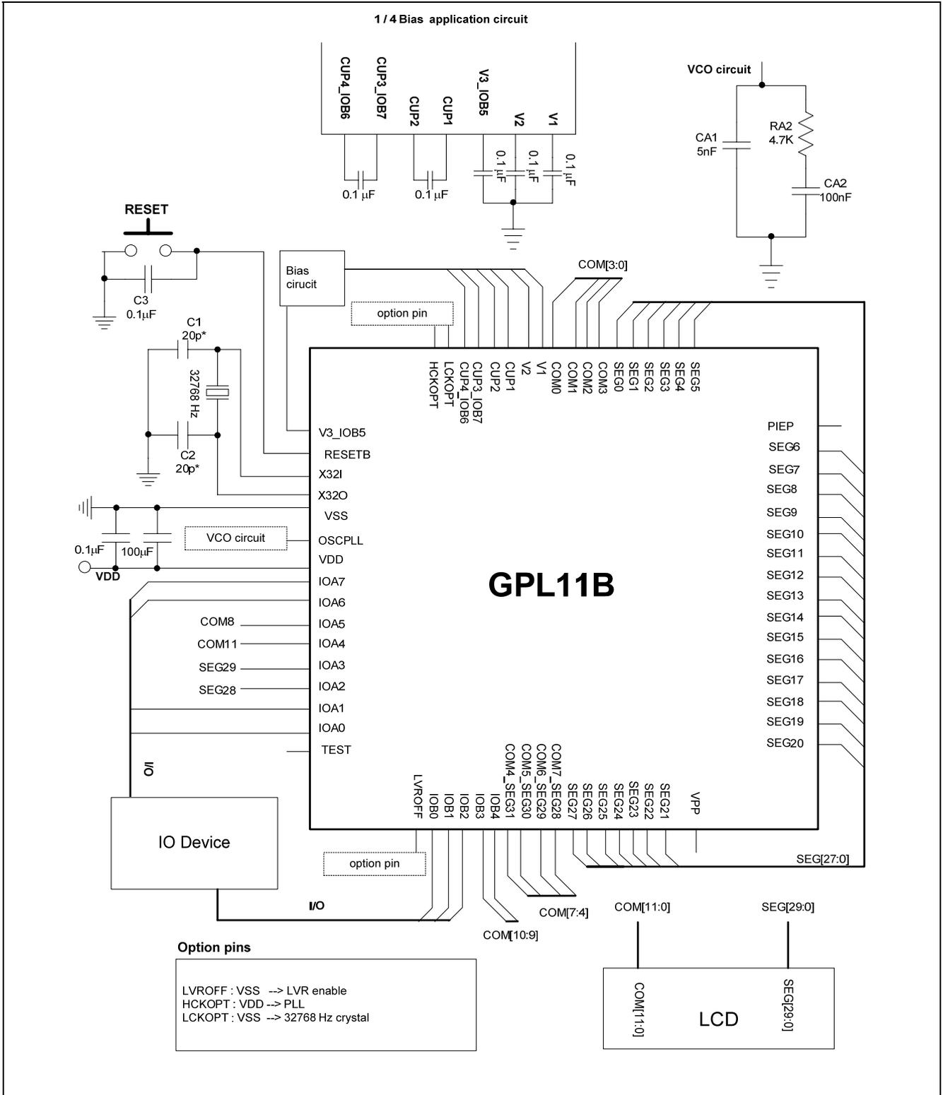
**Note\*:** C1/C2 values in above application circuit are for design guidance only. Different capacitor values may be required for different crystal used. Usually, the values of C1/C2 are in the range 12~20pF.
