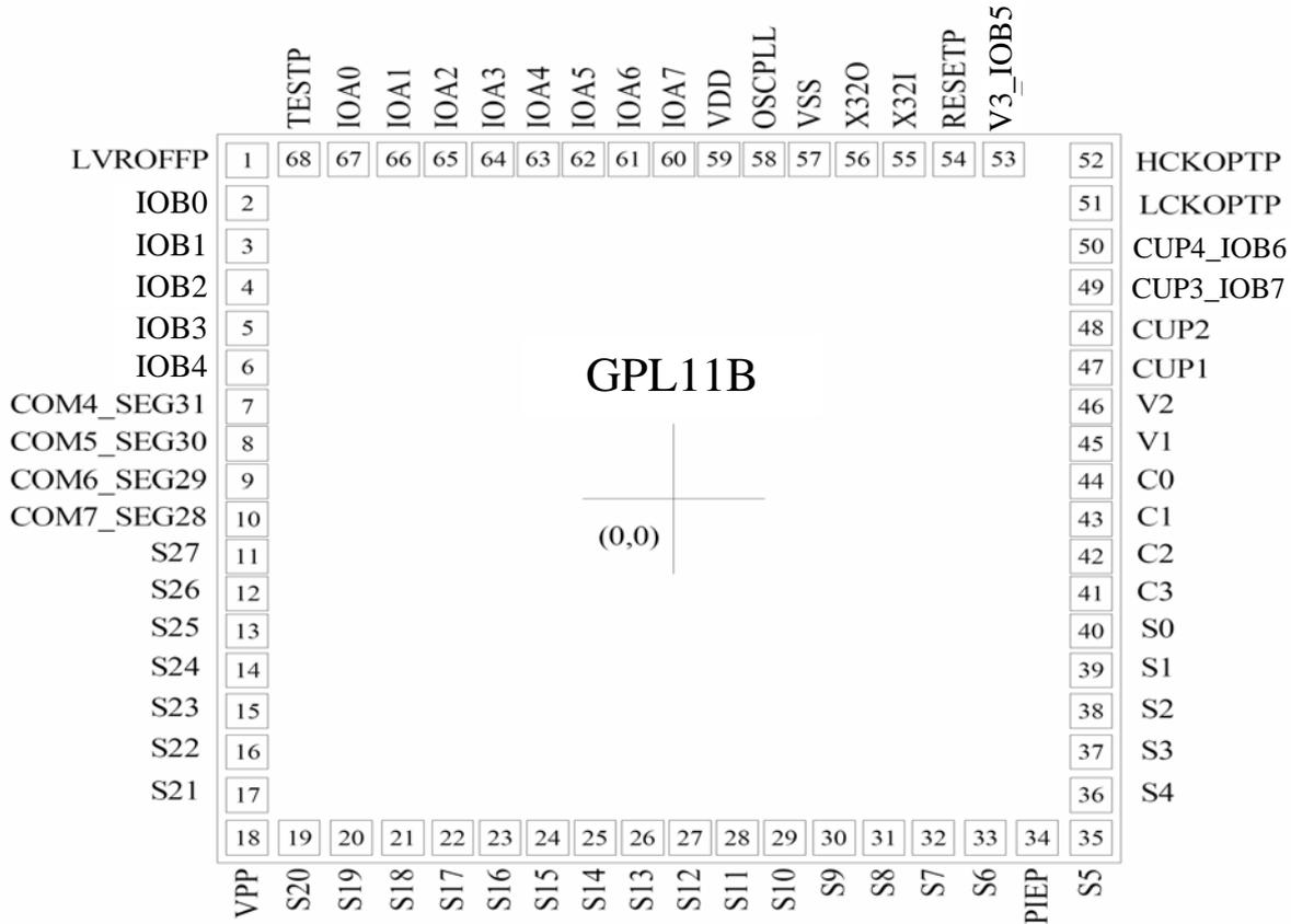
This IC substrate should be connected to VSS or floated
