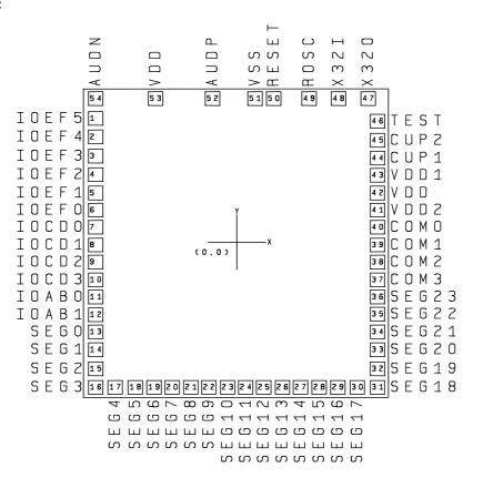
This IC substrate should be connected to VSS
