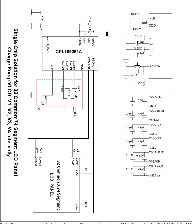
**Note\*1:** These capacitor values are for design guidance only. We recommend user select the ESR < 35K as well as CL1=CL=20~30pF(including PCB parasitic loading). Note that the environment humidity may affect the equivalent resistances on the two end points. To avoid the humidity effect, we recommend user to apply 20pF(assume PCB parasitic loading is 6pF) on XI and XO. Note that a larger CL capacitance will cause a longer time for XTAL to oscillate.
