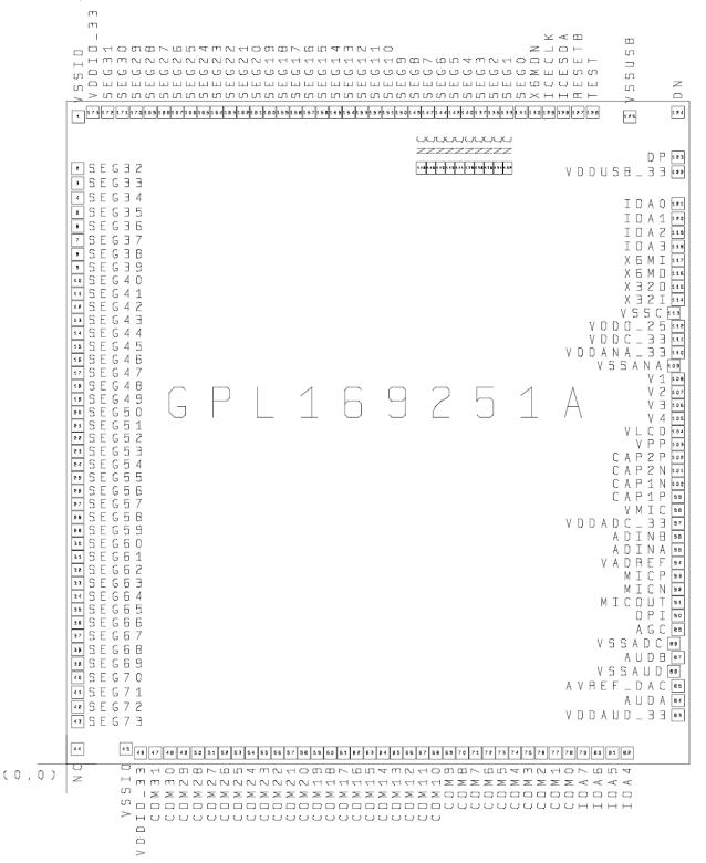
Note1: To ensure the IC functions properly, please bond all of VDD and VSS pins. Note2: The 0.1µF capacitor between VDD and VSS should be placed to IC as close as possible.
