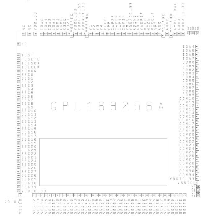
Note1: To ensure IC functions properly, please bond all of VDD and VSS pins.
