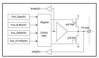
Although data can be written into the same register through Port\_Data and Port\_Buffer, they can be read from different places, Buffer (R) and Data (R). The IOA is software programmable for key wakeup capability. To activate key wakeup function, latch data on PORT\_IOA\_RL and enable the key wakeup function. Wakeup is triggered when the IOA state is different from at the time latched.
