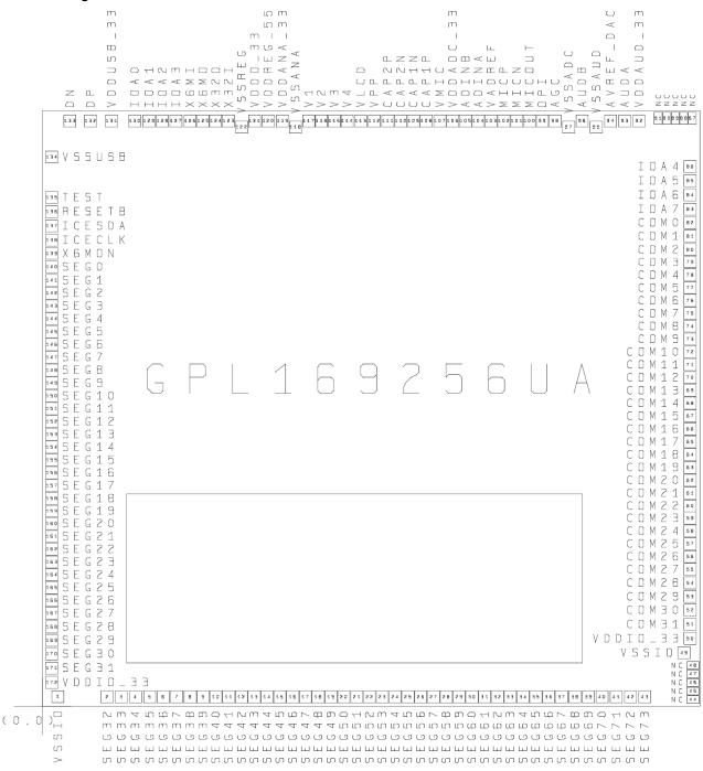
**Note1:** To ensure the IC functions properly, please bond all of VDD and VSS pins. **Note2:** The  $0.1\mu$ F capacitor between VDD and VSS should be placed to IC as close as possible.
