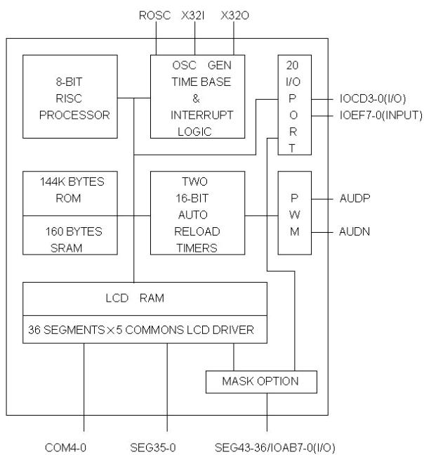
**Note:** IOAB7 - 0 can be mask option for segment 43 - 36. The mask option can be used as one I/O for one segment.
