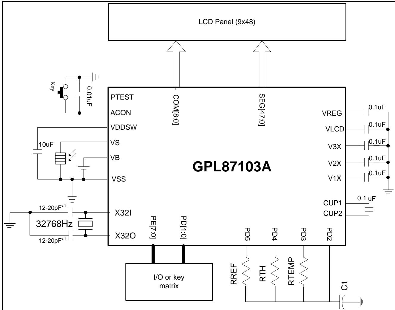
**Note1:** These capacitor values are for design guidance only. Different capacitor values may be required for different crystal/resonator used.
