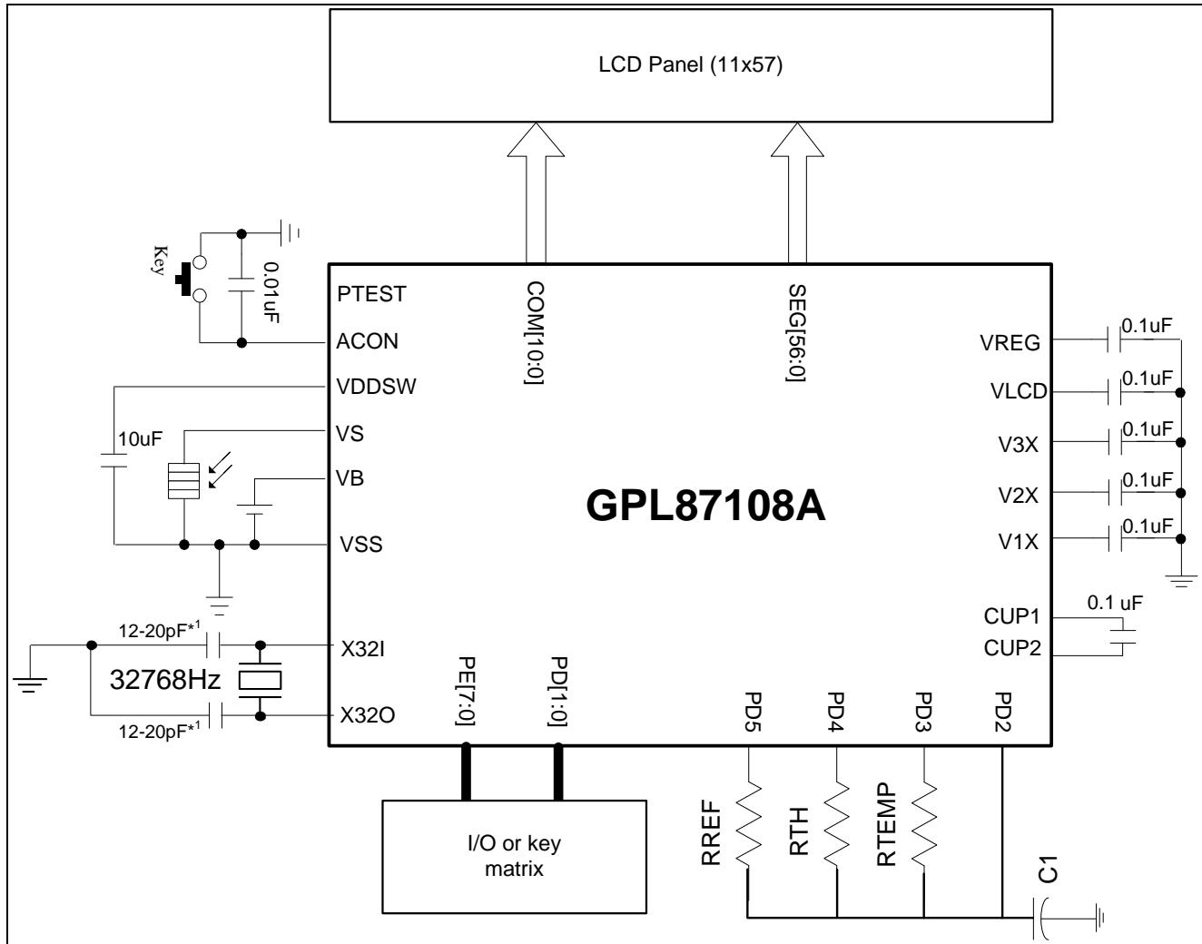
**Note:** These capacitor values are for design reference only. Different capacitor values may be required for different crystal/resonator used.
