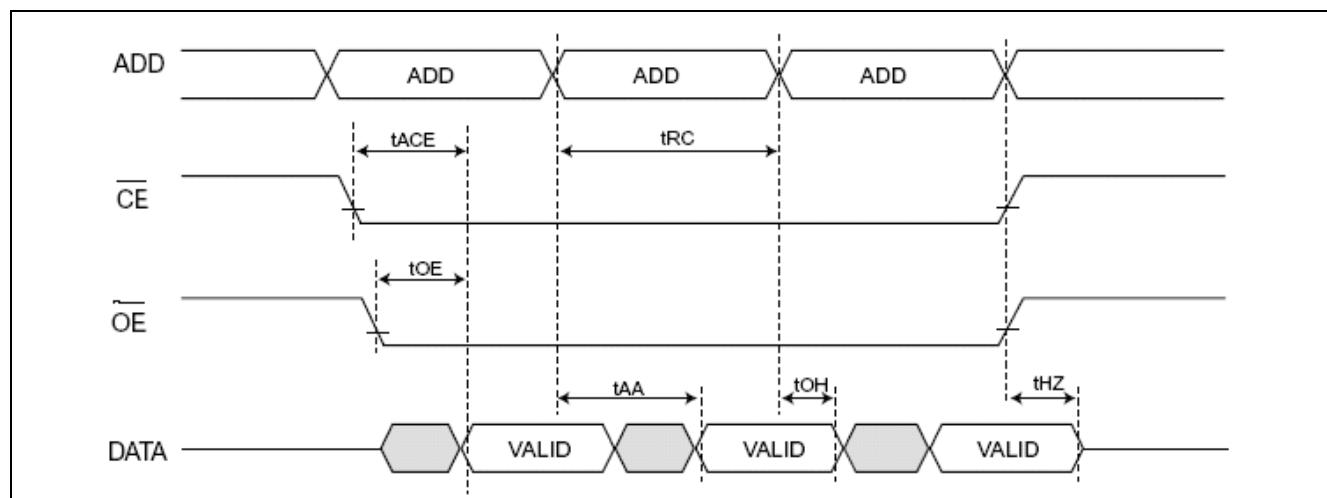
**\*Important Note:** It will fail to read 1st data from GPR23L800D after power on if CE is always set to ground level. Please refer the application note for further details.
