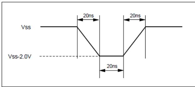
**Figure 40. Maximum Positive Overshoot Waveform**
