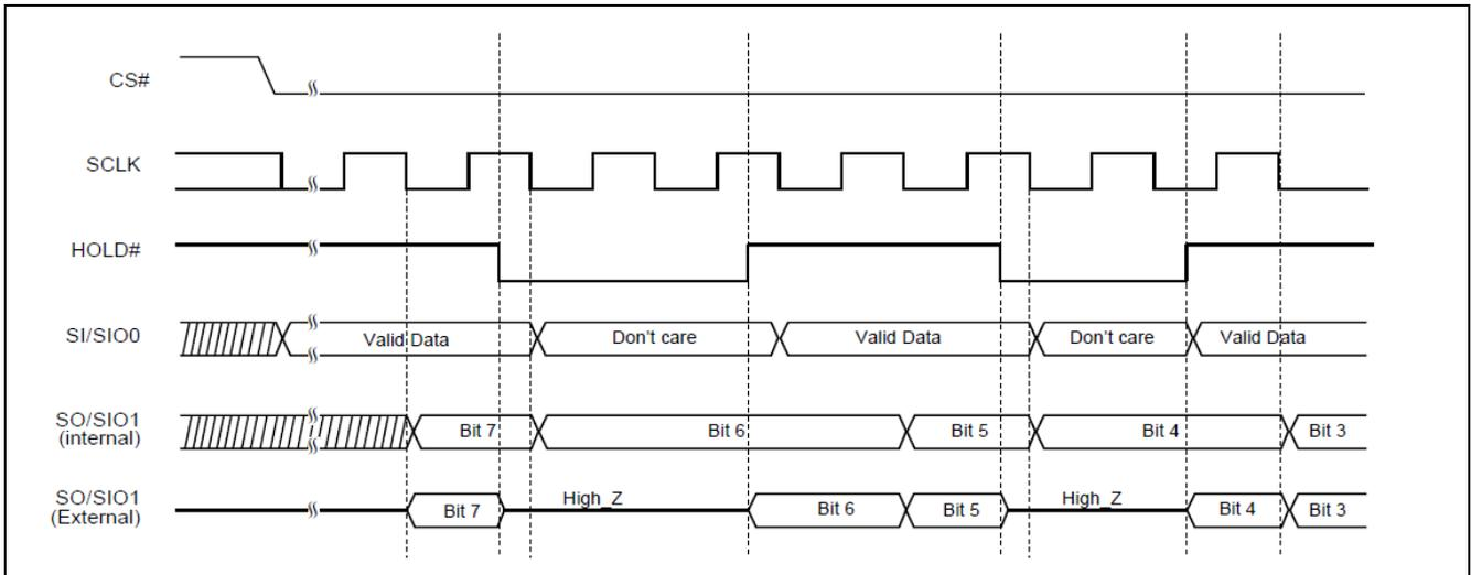
During the HOLD operation, the Serial Data Output (SO) is high impedance when Hold# pin goes low and will keep high impedance until Hold# pin goes high. The Serial Data Input (SI) is don't care if both Serial Clock (SCLK) and Hold# pin goes low and will keep the state until SCLK goes low and Hold# pin goes high. If
