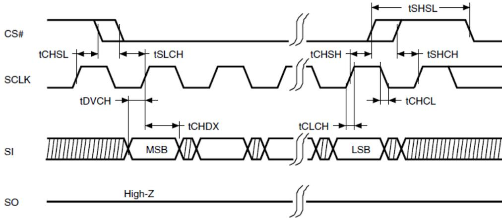
Figure 44. Output Timing
