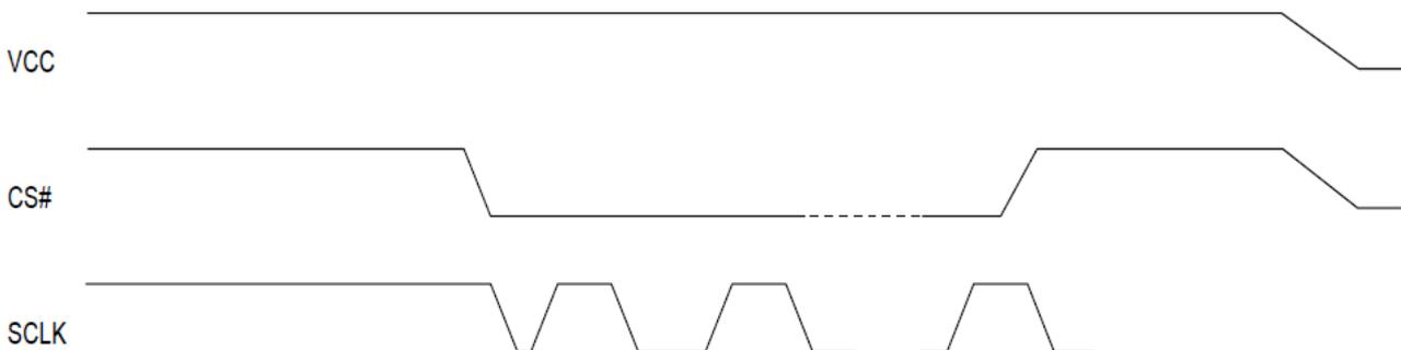
Figure 49. Power-up Timing
