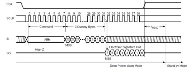
Figure 29. Release from Deep Power-down (RDP) Sequence
