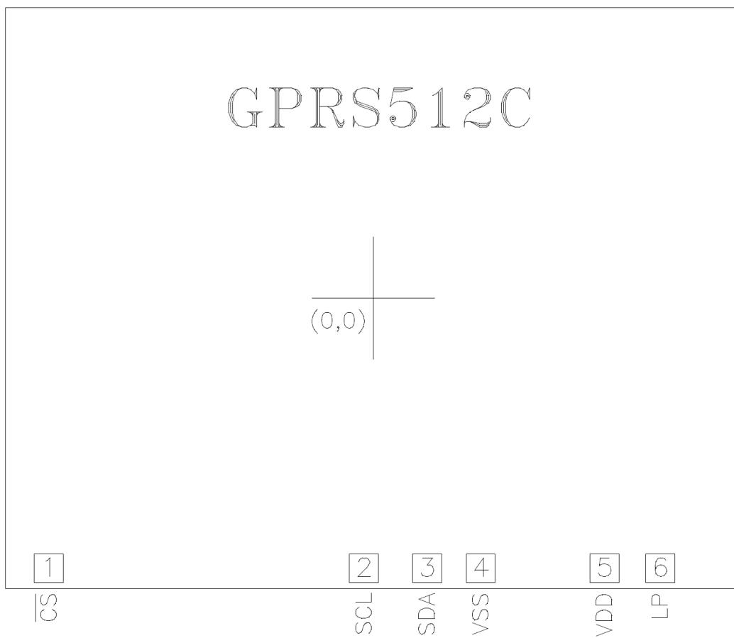
This IC substrate should be connected to VSS
