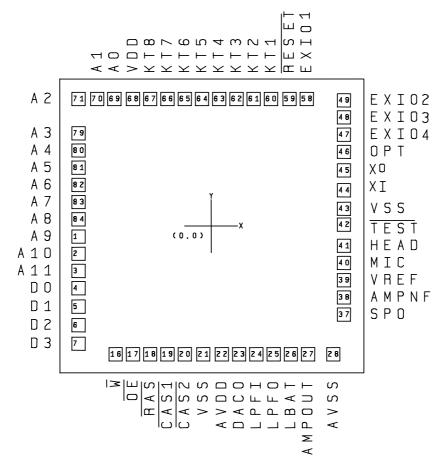
This IC substrate should be connected to VSS
