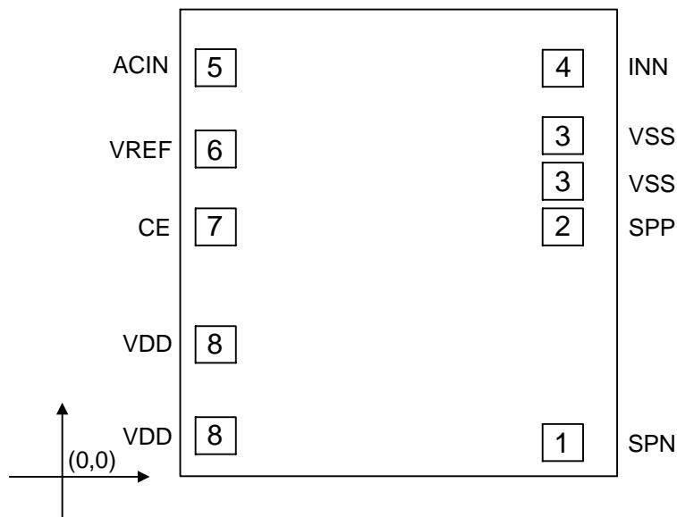
This IC substrate should be connected to VSS
