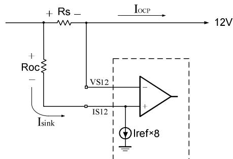
The recommended sense resistor values of RS12A, RS12B, RS5, and RS3 are  $\geq 0.002\Omega$  for good accuracy and enough SNR.
