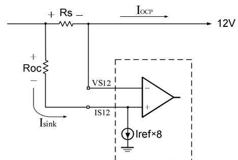
The recommend sense resistor values of RS12A, RS12B, RS5, and RS3 are  $\geq 0.002\Omega$  for good accuracy and enough SNR.
