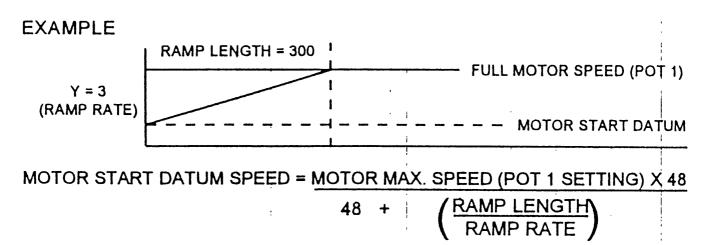
For the example above, if motor speed set at 400 step / second, MOTOR START DATUM SPEED =  $\frac{400 \times 48}{48 + 300} = \frac{19200}{148} = 130 \text{ Steps / Sec.}$
