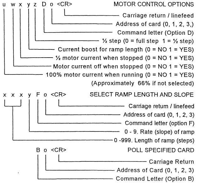
This command polls the card specified at address entered and returns an ID message plus limit switch status. e.g. B GSM4 999 JAN 95 L/F C/R or B GSM4 999 JAN 95 Limit Open L/F C/R
