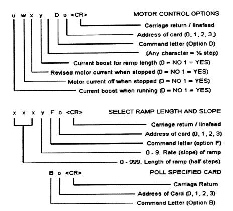
This command polls the card specified at address entered and returns an ID message plus limit switch status. e.g. B GSM5 999 JAN 95 L/F C/R or B GSM5 999 JAN 95 Limit Open L/F C/R
