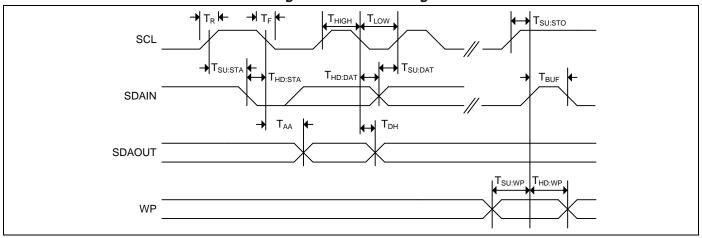
Figure 5-12. Write Cycle Timing
