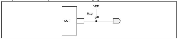
Toggle output mode is useful at lighting system on/off key switch application. For instance first touch can make light on output signal via OUT pin of the GT301L and this output signal maintains same light on states until next touch occurs.
