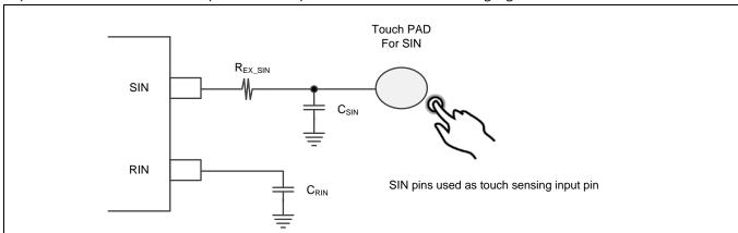
Implementation circuit for SIN pins and RIN pin is shown in the following figure.
