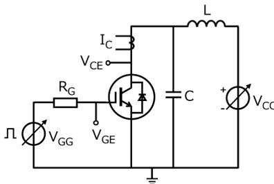
Fig. 6.2.3 Test Circuit of Switching Loss
