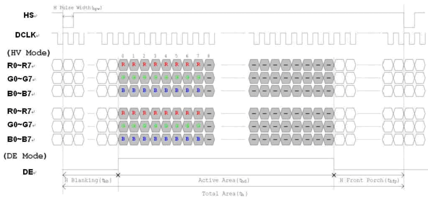
Figure 3. 1 Horizontal input timing diagram.
