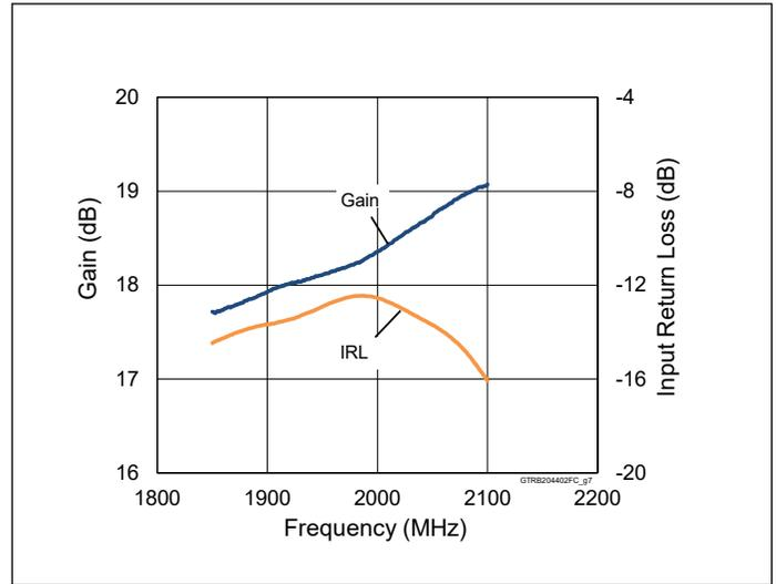
**Figure 6. Small Signal CW Gain & Input Return Loss**
