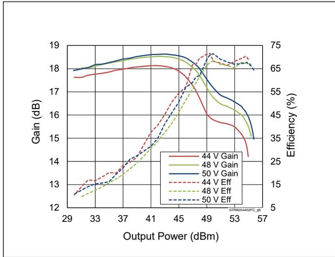
**Figure 5. Pulsed CW Performance at various  $V_{DD}$**
