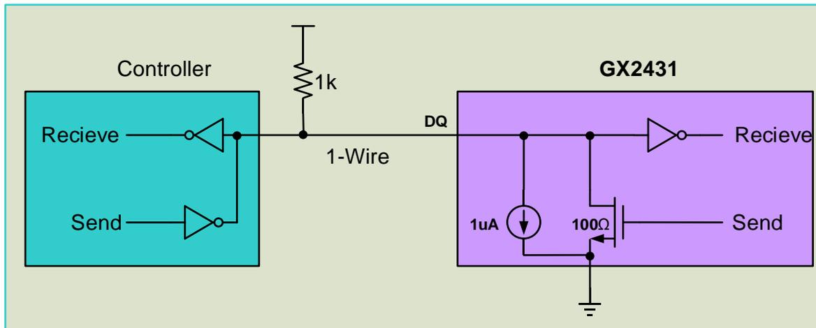
**Figure 6. Hardware Configuration**
