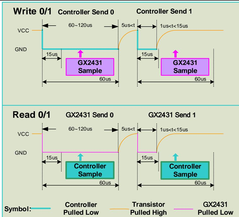
**Figure 10. Read/Write Time Slot Timing Diagram**
