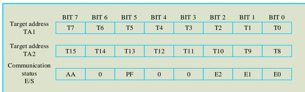
**Figure 4. The GX2431 Address Registers**
