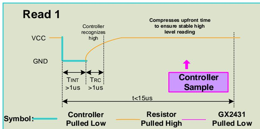
Figure 12. Recommended Controller 1 Timing
