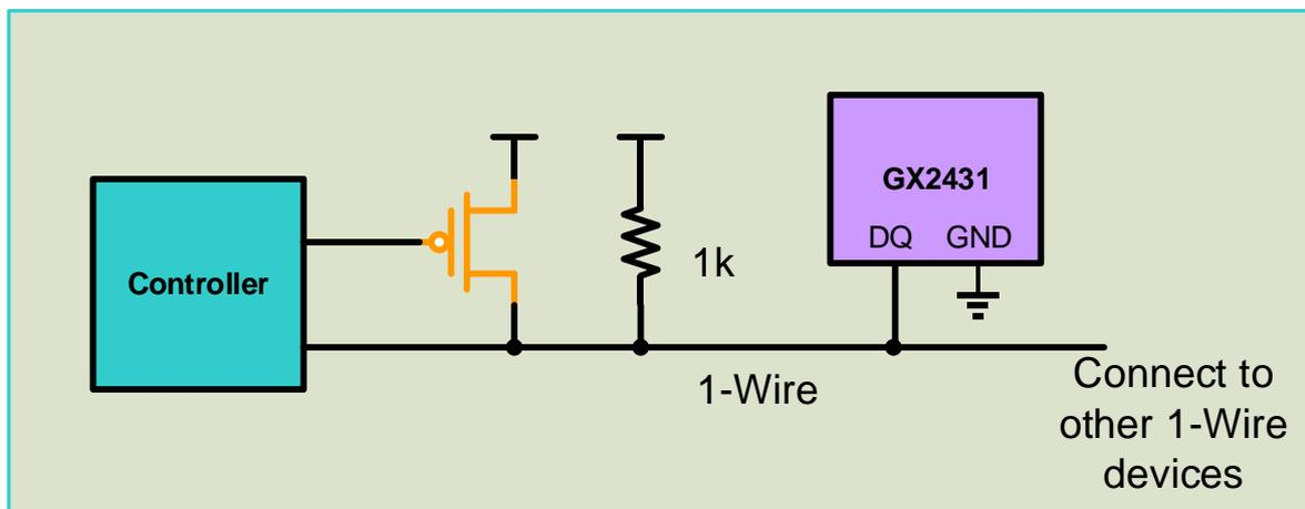
Figure 2. Parasitic Mode Replicated Data Circuit
