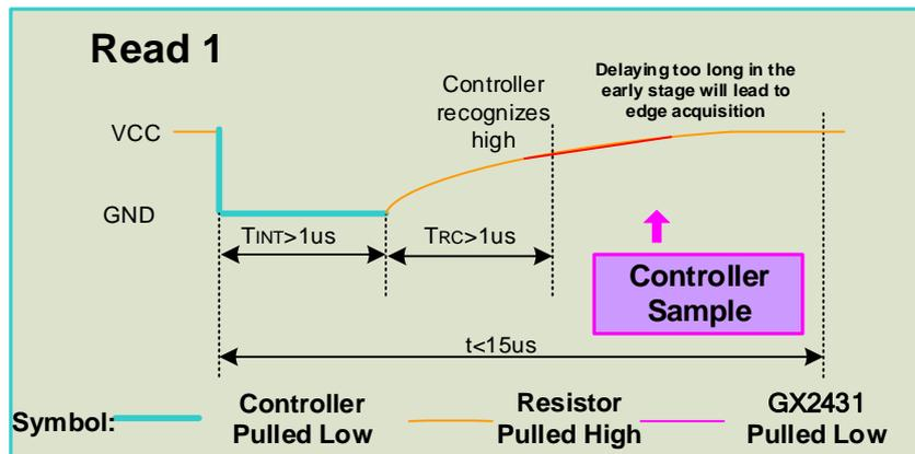
Figure 11. Detailed Timing of Controller Read 1
