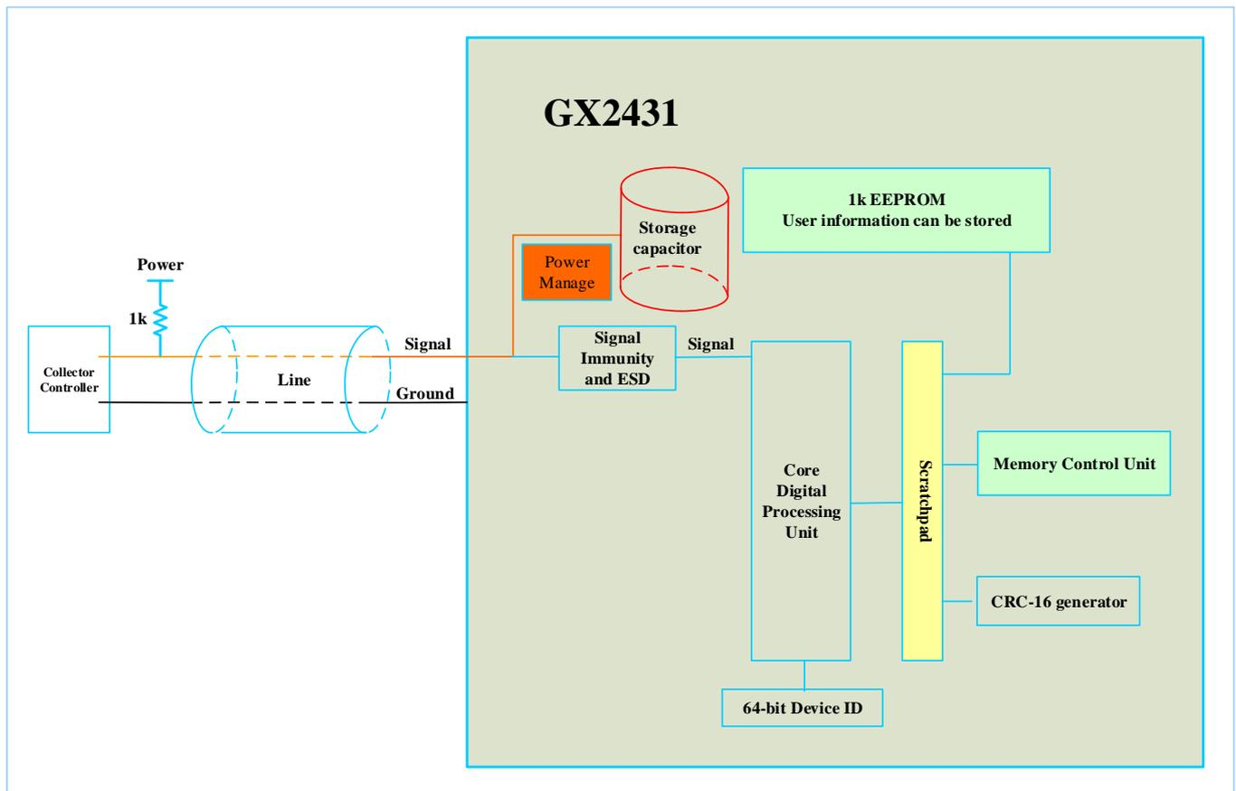
**Figure 1. The GX2431 Block Diagram**
