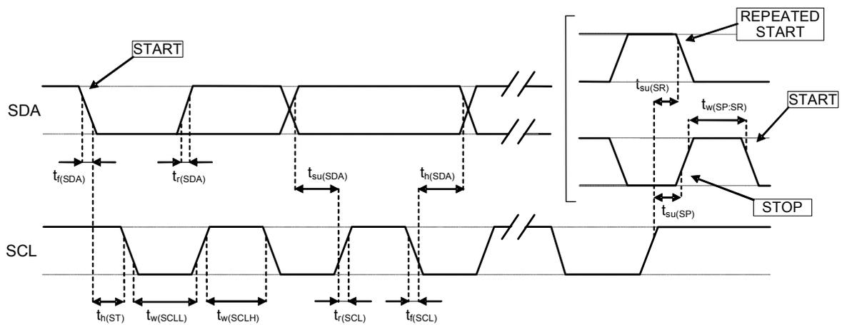
*Note:* Measurement points are done at 0.2·V<sub>dd\_IO</sub> and 0.8·V<sub>dd\_IO</sub> for both ports.
