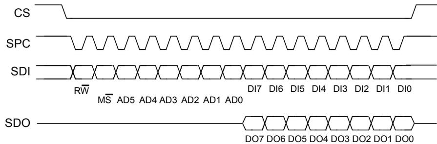
**CS** enables the serial port and it is controlled by the SPI master. It goes low at the start of the transmission and goes back high at the end. **SPC** is the serial port clock and it is controlled by the SPI master. It is stopped high when **CS** is high (no transmission). **SDI** and **SDO** are respectively the serial port data input and output. Those lines are driven at the falling edge of **SPC** and should be captured at the rising edge of **SPC**.
