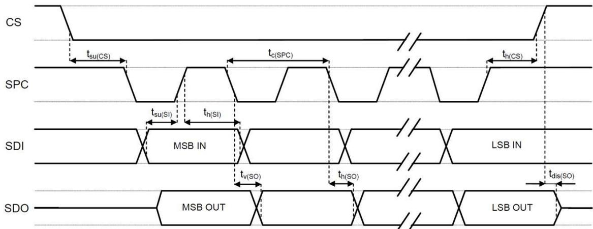
Note: Measurement points are done at  $0.2 \cdot V_{dd\_IO}$  and  $0.8 \cdot V_{dd\_IO}$  for both input and output ports. When no communication is ongoing, data on CS, SPC, SDI, and SDO are driven by internal pull-up resistors.
