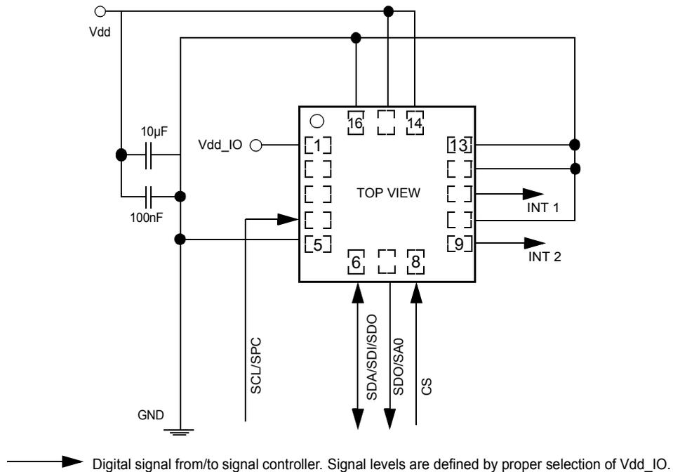
The device core is supplied through the Vdd line while the I/O pins are supplied through the Vdd\_IO line. Power supply decoupling capacitors (100 nF ceramic, 10 µF aluminum) should be placed as near as possible to pin 14 of the device (common design practice).
