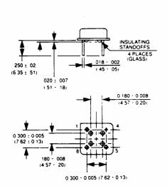
Pin number 4 connected to case.
