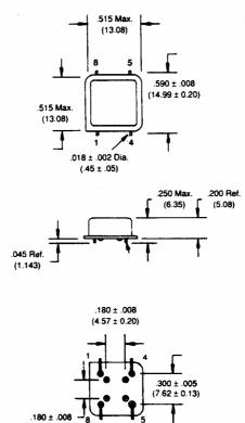
Pin number 4 connected to case. Seating plane = .005 Max. (.127) Wire leads to be formed to a 90° angle.
