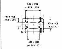
Pin number 7 connected to case. Seating plane = .005 Max. (.127) Wire leads to be formed to a 90° angle.
